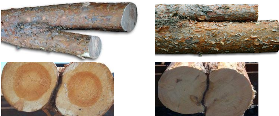
Open fork – air between fork limb and the main stem
